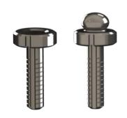
Post length: 7 mm Ø base: 3.4 mm Ø post: 1.35 mm Threads: M 2 Ø ball: 2,25 mm
